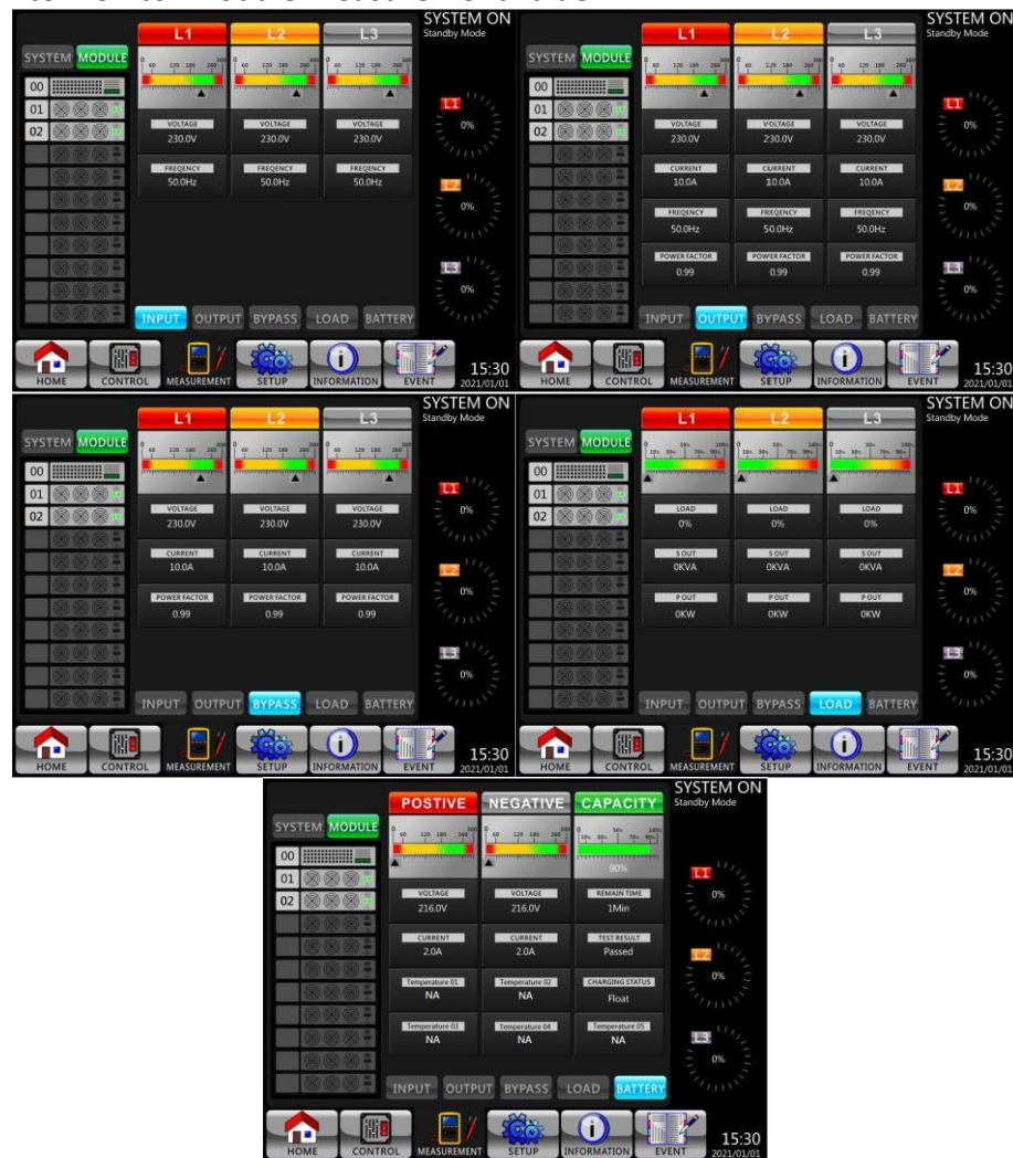
Figure 4-10 Module Measurement Screens
