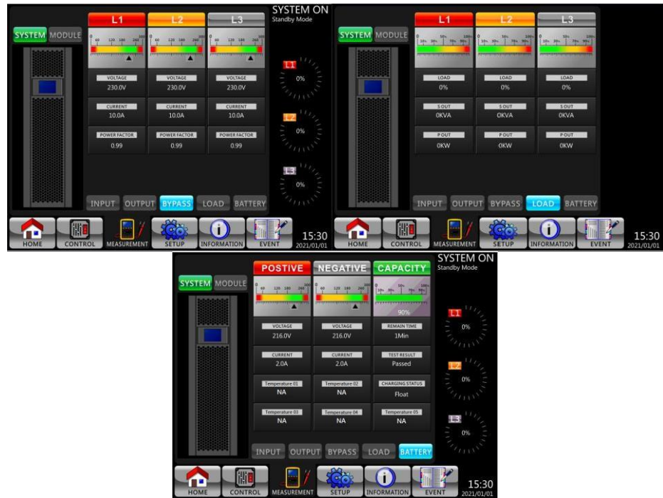
Figure 4-9 System Measurement Screens
